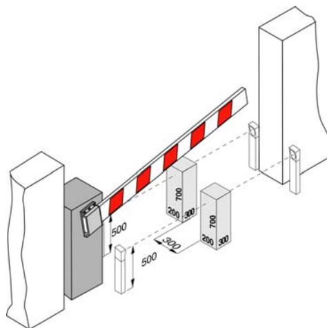
**[5] Shearing, dragging and cutting between the bar and the drive unit (Figure 1, risk B).**
