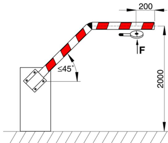
The graph indicates the maximum values of the dynamic, static and residual operating forces in relation to the various positions of the bar.
